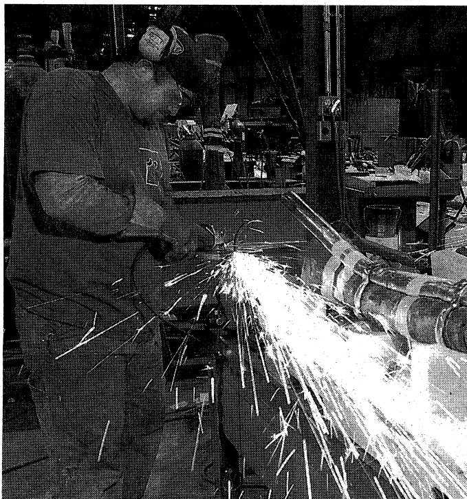
Brett Crawford works on the fabrication of steel armatures for the Barosaurus exhibit. TIBOR KOLLEY/THE GLOBE AND MAIL
